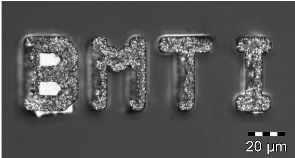
Figure 3.16 Light microscopy image (in reflection), showing the versatility of the described delayed lift-off method. The electroplated cobalt structures shown are composed of lines of 11\mu\text{m} width, and have a thickness of 6\mu\text{m} . The area surrounding the structures is bare glass. For very small enclosed structures, it can be difficult to remove the resist and seed layer. This can be seen in the letter 'B' where the platinum seed layer is still present, which creates the strong reflection.
